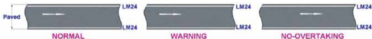
Fig. 4.13 Single/Intermediate Lane Ramp/Slip Road/One Way Street (Paved Width upto 5.5 m)
