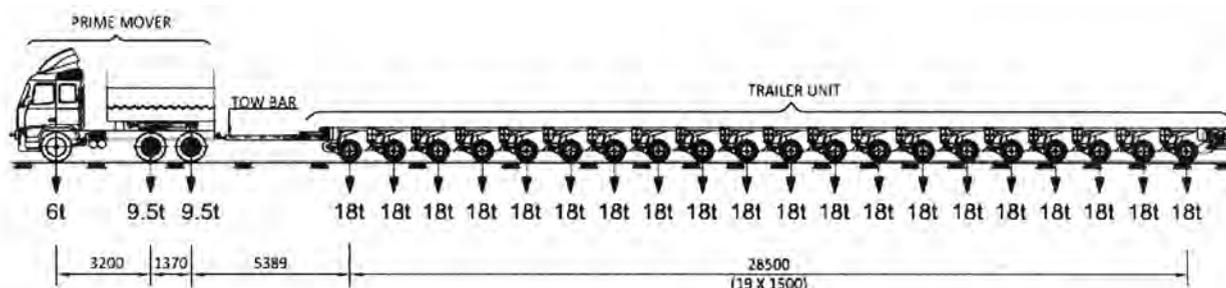
**Fig. 6: Typical Axle Arrangement for Special Vehicle**
