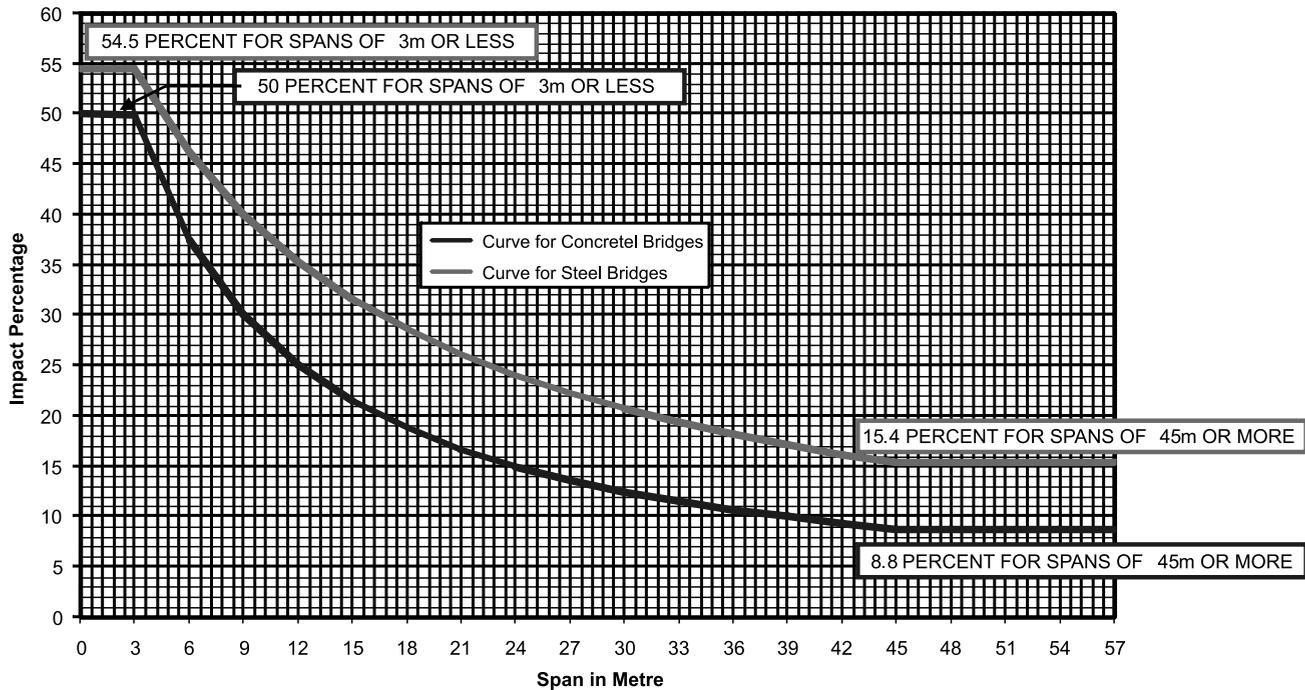
**Fig.9: Impact Percentage for Highway Bridges for Class A and Class B Loading (Clause 208.2)**
