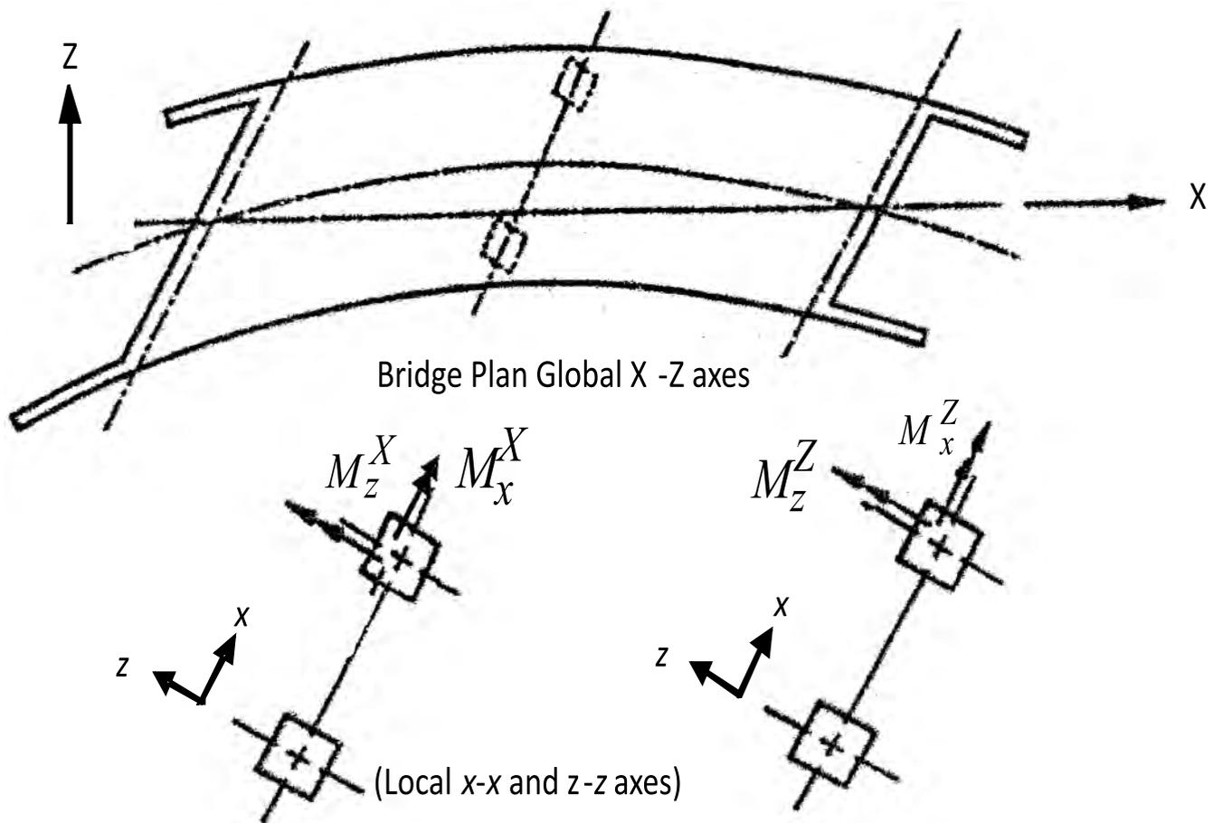
Fig. 18: Combination of Orthogonal Seismic Forces
