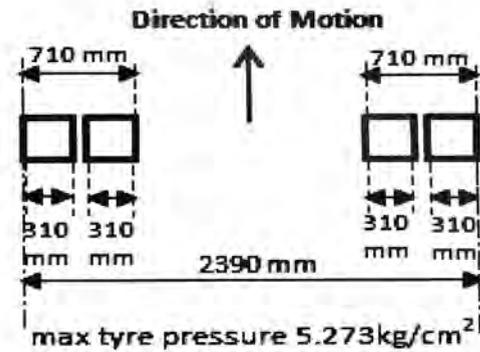
Fig. 7B: Transverse Wheel Spacing and Tyre Arrangement
