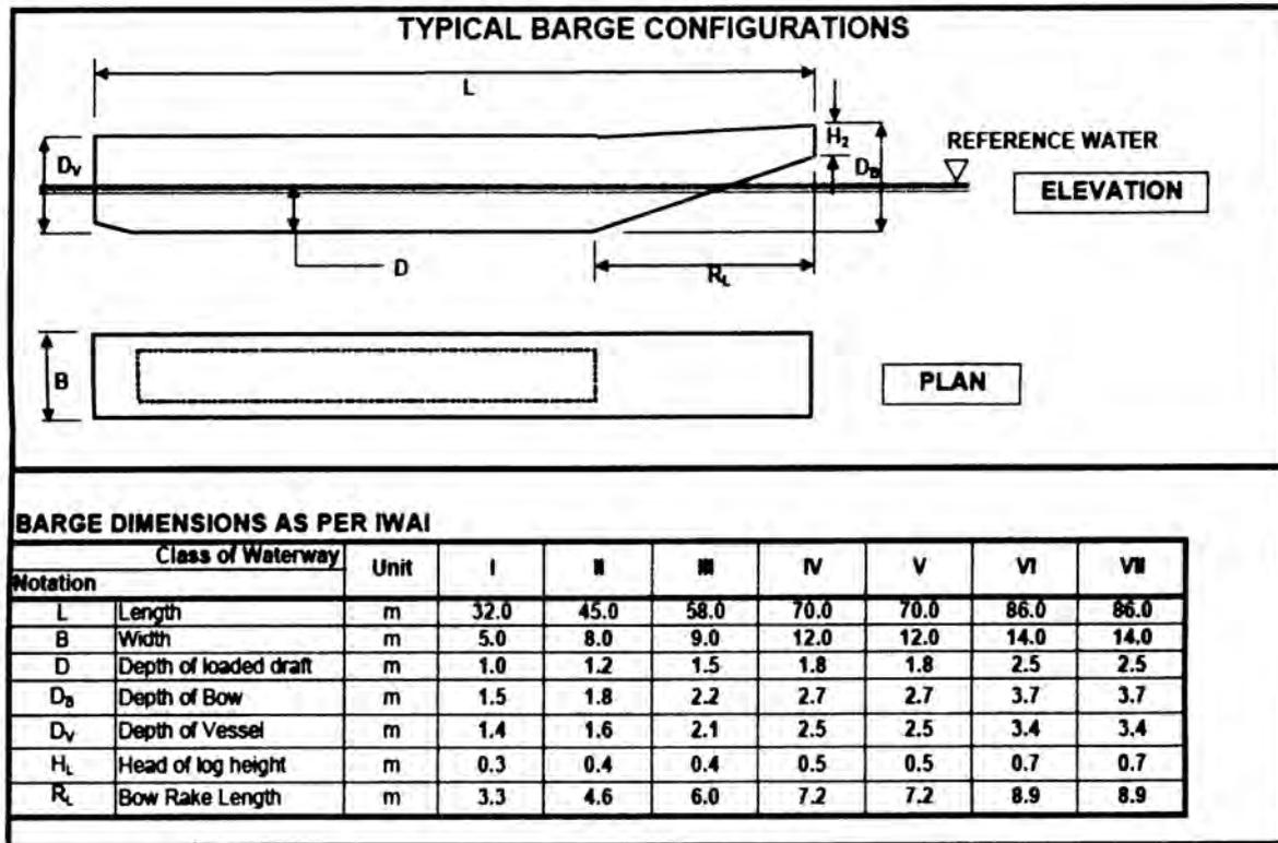
Fig. 23: Typical Barge Dimensions
