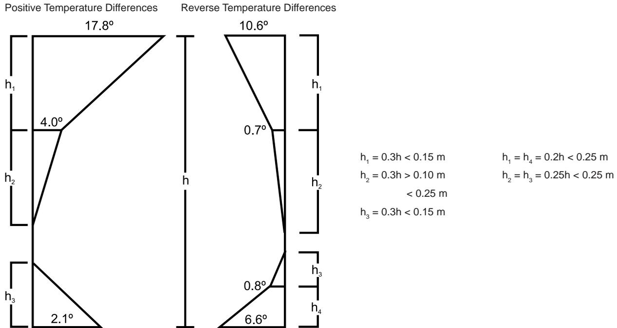
Fig. 16a: Design Temperature Differences for Concrete Bridge Decks
