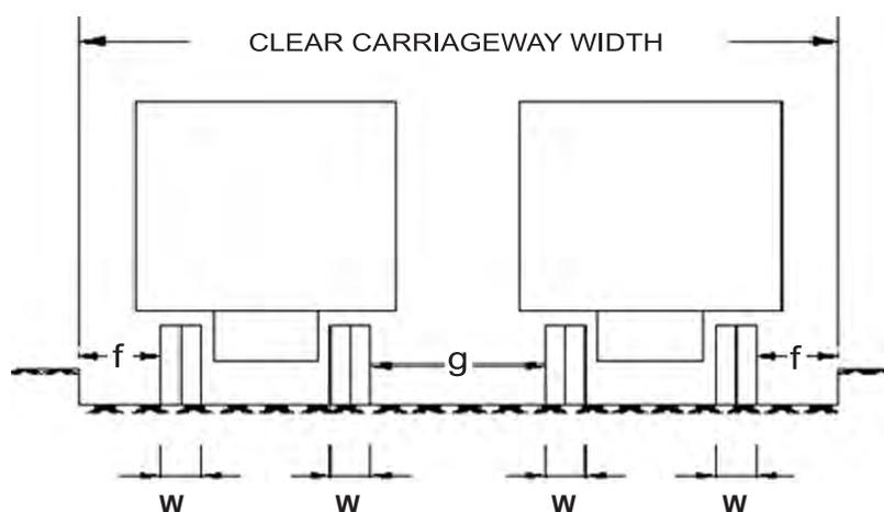
**Fig. 5: Minimum Clearance for 2 Class B Train**
