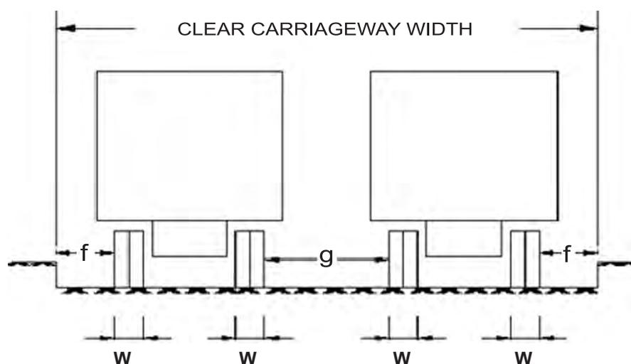
**Fig. 3: Minimum Clearance for 2 Class A Train Vehicles**
