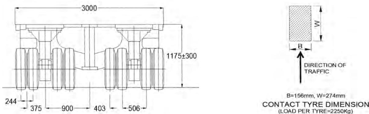
**Fig. 6A: Transverse Wheel Spacing of Special Vehicle**
