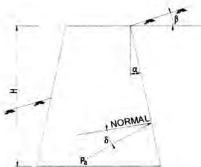
**Fig.13A: Diagram for Active Earth Pressure**
