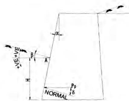
**Fig.13B: Diagram for Passive Earth Pressure**
