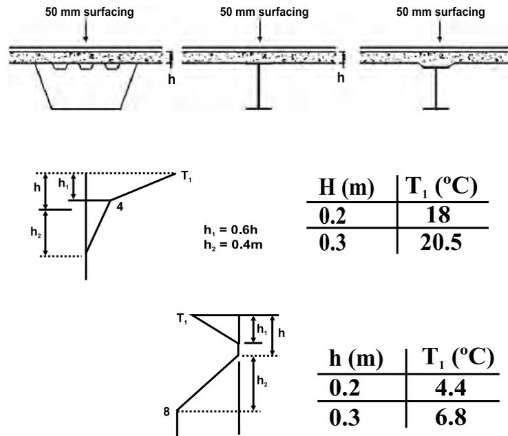
Fig. 16b: Temperature Differences Across Steel and Composite Section
