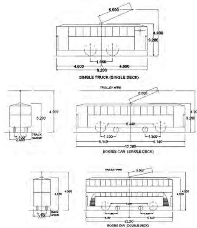
**Fig. 8: Average Dimension of Tramway Rolling Stock (Clause 207.1)**
