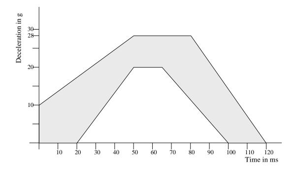
FIG 4 SLED DECELERATION AS A FUNCTION OF TIME (Para 5.3.1) (Frontal Impact)
