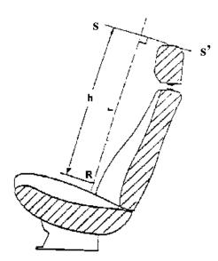
R = Reference Point r = Reference Line h = Height s-s'=Line drawn perpendicular to the reference line passing through the top most point of head restraint.
