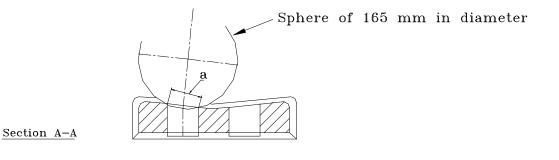
Fig 3 Example of Vertical Gaps(Para 4.6.2 :
