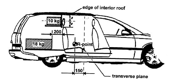
FIG 8 TESTING OF A PARTITIONING SYSTEM ABOVE THE BACK REST (Para 5.9.3)
