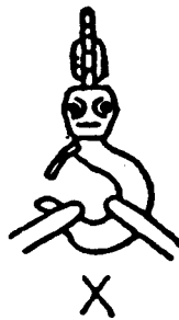
2. Sling load from the centre of the hook
