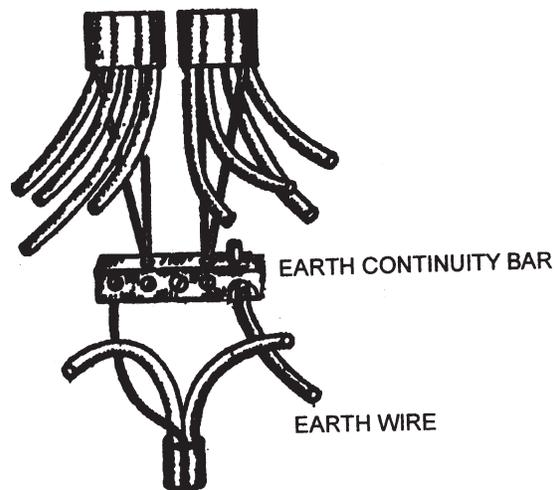
FIG. 31 EARTH CONTINUITY BAR AND ARRANGEMENT FOR CONNECTION OF EARTH WIRES OF DIFFERENT CIRCUITS
