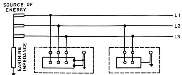
NOTE — All exposed conductive parts of an installation are connected to an earth electrode.
