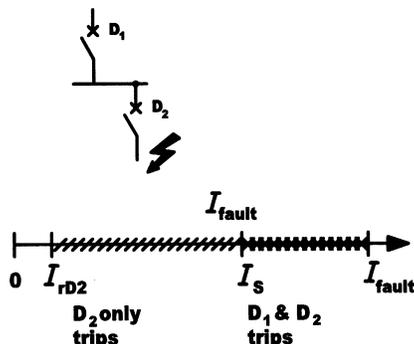
FIG. 16 DISCRIMINATION AND SEQUENCE OF TRIPPING
