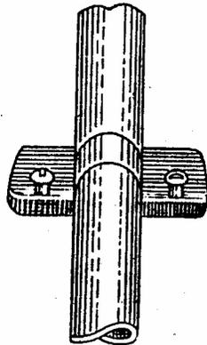
FIG. 40 INSTALLATION OF CONDUIT WITH SPACING SADDLE
