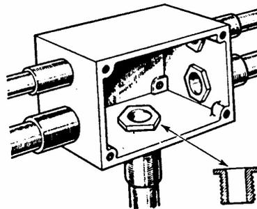
NOTE — Where two or more conduits are run in parallel it is good practice to embrace all conduits with an adaptable box.
