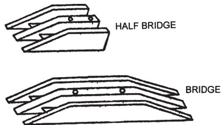
FIG. 22 HALF BRIDGE AND BRIDGE
