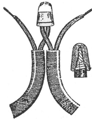
FIG. 27 WIRES CONNECTED WITH THIMBLE
