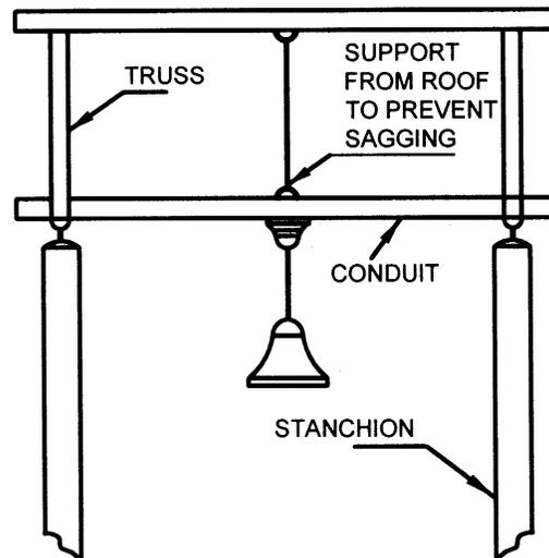
FIG. 45 A CONDUIT SUSPENDED ACROSS ROOF TRUSSES
