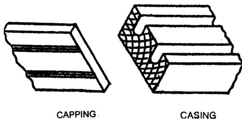
FIG.14 WOODEN CAPPING AND CASING
