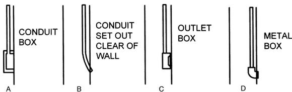
NOTE — A box or suitable enclosure must be fitted at all outlet positions. Terminations as shown at B, C and D are not permitted.
