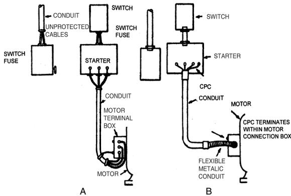
NOTE — Figure 49A shows the wrong method, which is frequently adopted because proper conduit outlets are not always provided on starters and motors. The lengths of unprotected cable are subject to mechanical damage which may lead to electrical breakdown. Figure 49B illustrates the right method. Conduit is either taken direct into the equipment or terminated with flexible metallic conduit and a suitable c.p.c.
