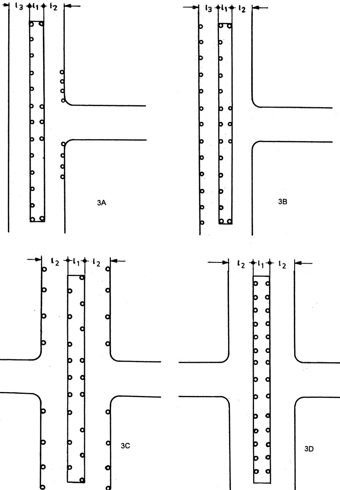
FIG. 3 STANDARD LAYOUTS FOR FLYOVERS (FOUR ALTERNATIVES)
