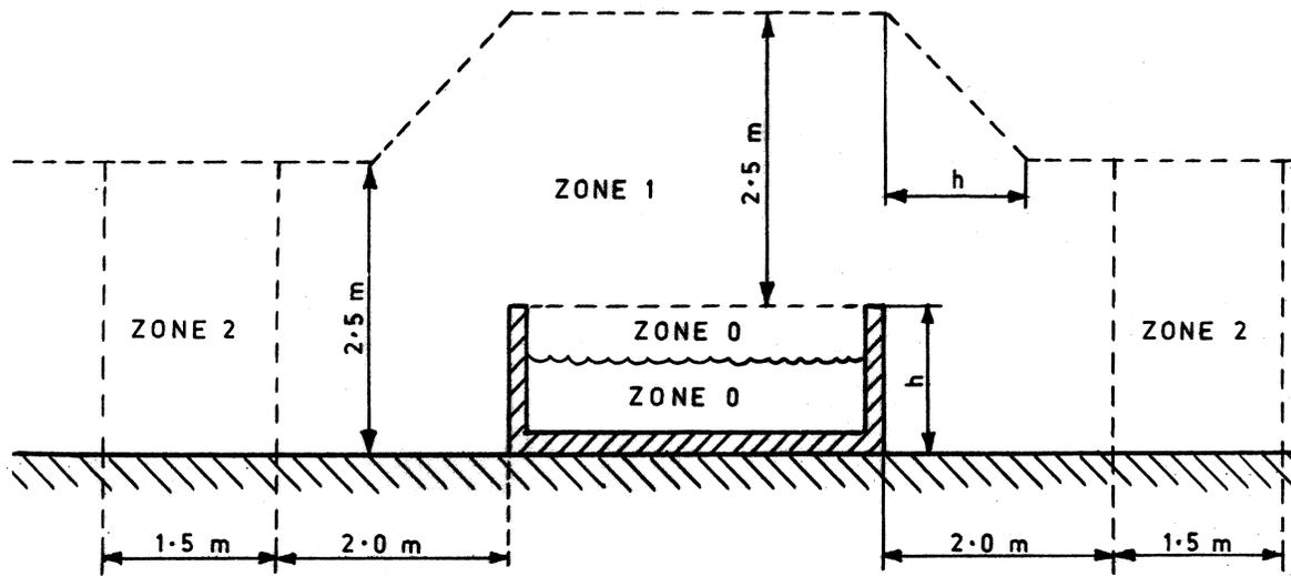
FIG. 1 ZONE DIMENSIONS FOR BASINS ABOVE GROUND
