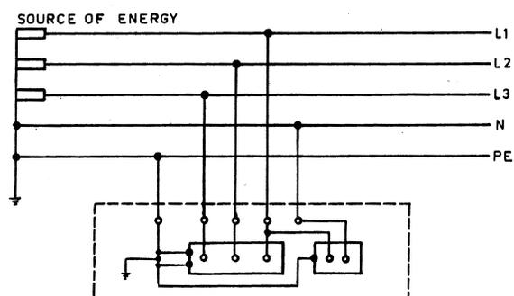
NOTE — For 415 V Three Phase Domestic/Commercial Supply Having 3-Phase and 1-Phase Loads. All exposed conductive parts of the installation are connected to protective conductor via the main earthing terminal of the installation. An independent earth electrode within the consumer's premises is also provided.
