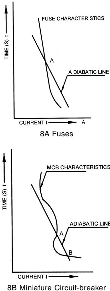
FIG. 8 RELATIONSHIP BETWEEN ADIABATIC LINES AND CHARACTERISTICS
