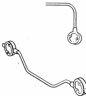
NOTE — Cable must not be drawn round more than two right angle bends or their equivalent. The four bends in the lower diagram are each 45° making a total of 180° in all.
