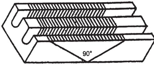
FIG. 19 HOW A SMALL PIECE OF CASING IS OBTAINED FOR A CORNER JOINT
