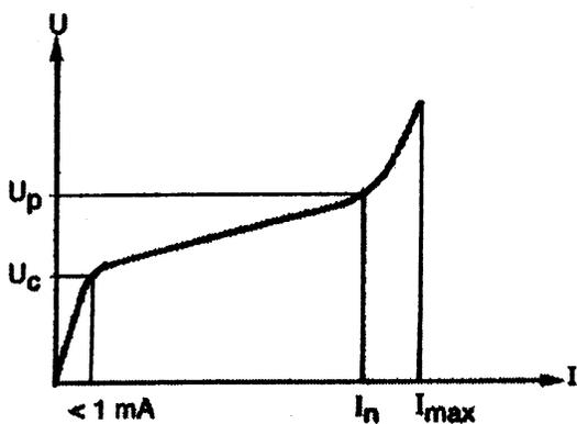
FIG. 3 VOLTAGE/CURRENT CHARACTERISTICS
