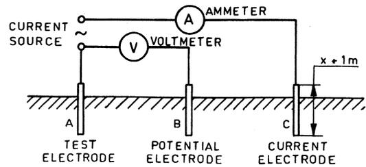
FIG. 5 METHOD OF MEASUREMENT OF EARTH ELECTRODE RESISTANCE
