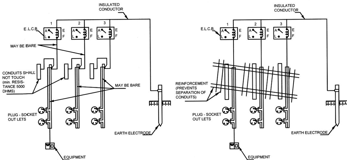
10A Complete Separation of the Exposed Metal of One Installation from that of Other Installation
