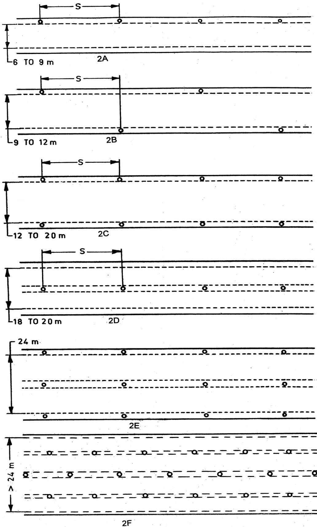
FIG. 2 STANDARD LAYOUTS FOR ROADS (SIX ALTERNATIVES)
