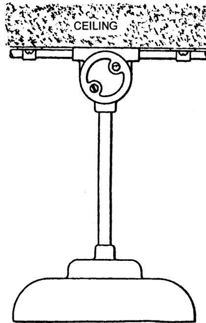
NOTE — The conduit is fixed to the ceiling with spacer bar saddles.
