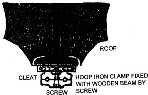
FIG. 10 ARRANGEMENT FOR DRAWING WIRES UNDER IRON BEAM
