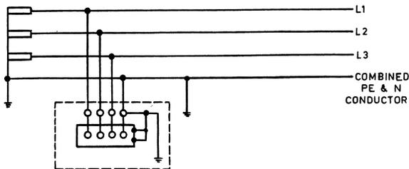
NOTE — The usual form of a TN-C-S system is as shown, where the supply is TN-C and the arrangement in the installations in TN-S. This type of distribution is known also as Protective Multiple Earthing and the PEN conductor is referred to as the combined neutral and earth (CNE) conductor.
