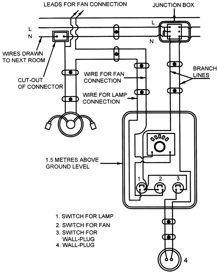
FIG. 12 AN EXAMPLE OF CLEAT WIRING SYSTEM
