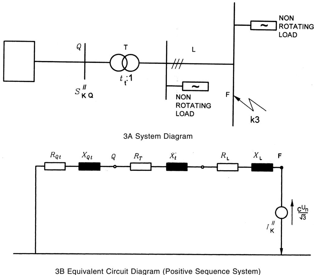
FIG. 3 ILLUSTRATION FOR CALCULATING THE INITIAL SYMMETRICAL SHORT-CIRCUIT CURRENT  $I''_k$  IN COMPLIANCE WITH THE PROCEDURE FOR THE EQUIVALENT VOLTAGE SOURCE
