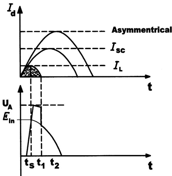
FIG. 13 EFFECT OF LIMITATION ON FAULT CURRENT
