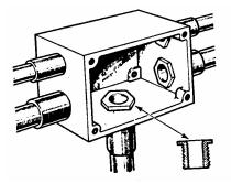
NOTE — Where two or more conduits are run in parallel it is good practice to embrace all conduits with an adaptable box.
