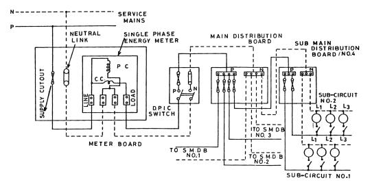
FIG. 2 TYPICAL HOUSE-WIRING CIRCUIT
