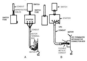
NOTE — Figure 49A shows the wrong method, which is frequently adopted because proper conduit outlets are not always provided on starters and motors. The lengths of unprotected cable are subject to mechanical damage which may lead to electrical breakdown. Figure 49B illustrates the right method. Conduit is either taken direct into the equipment or terminated with flexible metallic conduit and a suitable c.p.c.
