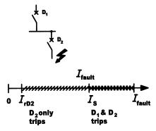
FIG. 16 DISCIMINATION AND SEQUENCE OF TRIPPING
