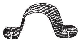
FIG. 37 Spacing Saddles with Oval Holes
