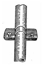
Fig. 40 Installation of Conduit with Spacing Saddle
