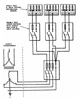
NOTE — When the neutral point of a supply or one pole of transformer on consumer's premises is earthed permanently, a fuse, nonlinked switch or circuit-breaker is not permitted in the line connected to earth.
