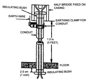
Fig. 26 Leading of Cable Through the Floor
