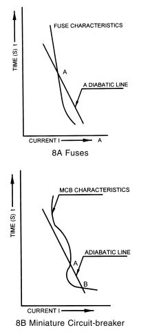
FIG. 8 Relationship Between Adiabatic Lines and Characteristics
