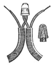
FIG. 27 WIRES CONNECTED WITH THIMBLE
