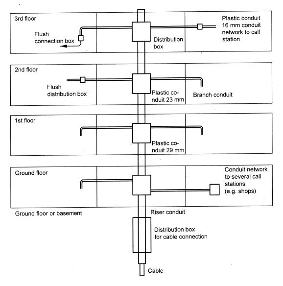
FIG. 5 TYPICAL CONDUIT WIRING SYSTEM
