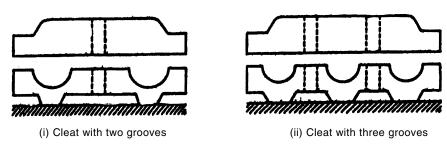
iron beam, at first pieces of wood are clamped at intervals to the bottom of the beam and then the cleats are fixed on these wood pieces. This is shown in Fig. 10. The spacing between two consecutive pieces of wood should be such that the wiring must not sag due to its own weight. If wiring is to be taken from one room into the next, a hole is drilled into the common wall and wiring is taken through porcelain or metal tube (wall-tube) set into the hole.
