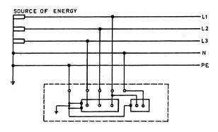
NOTE — For 415 V Three Phase Domestic/Commercial Supply Having 3-Phase and 1-Phase Loads. All exposed conductive parts of the installation are connected to protective conductor via the main earthing terminal of the installation. An independent earth electrode within the consumer's premises is also provided.
