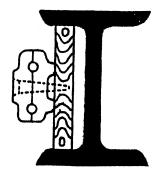
FIG. 9 CLEAT IS FIXED ON AN WOOD PIECE WHICH IS TIGHTLY ATTACHED ON ONE SIDE OF AN IRON BEAM
