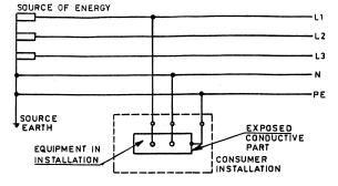
NOTE — The protective conductor (PE) is the metallic covering (armour or load sheath of the cable supplying the installation or a separate conductor). All exposed conductive parts of an installation are connected to this protective conductor via main earthing terminal of the installation.
