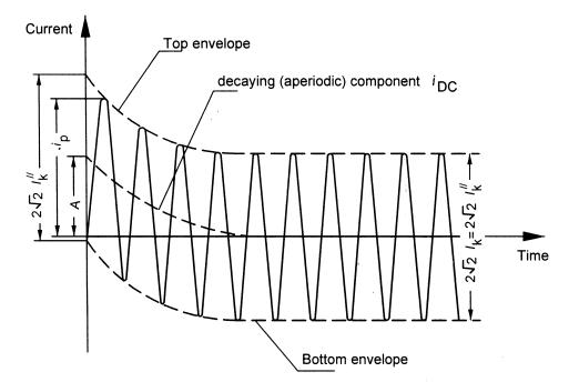
FIG. 1 SHORT-CIRCUIT CURRENT AT A SYSTEM FAR-FROM-GENERATOR
