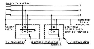
NOTE — All exposed conductive parts are connected to the PEN conductor. For 3~ consumer, local earth electrode has to be provided in addition.
