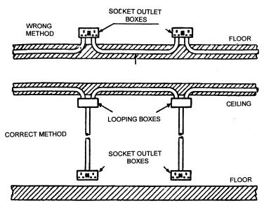
NOTE — If the sockets are fed from the floor below, it is difficult to avoid a trap for moisture.
