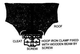
Fig. 10 Arrangement for Drawing Wires Under Iron Beam
