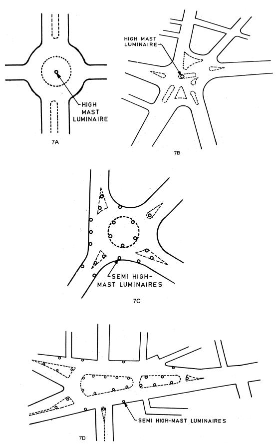
FIG. 7 USE OF HIGH MAST, SEMI-HIGH-MAST LUMINAIRES IN ROUNDABOUTS (FOUR ALTERNATIVES)
