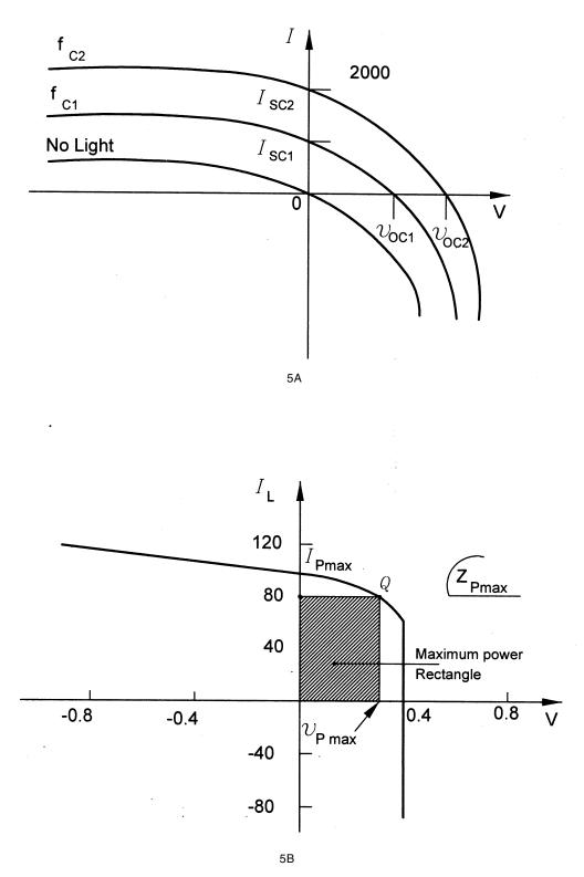
FIG. 5 CURRENT-VOLTAGE CHARACTERISTICS OF A PV CELL
