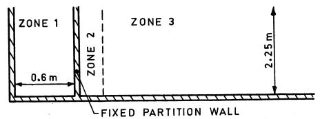
FIG. 1 ZONE DIMENSIONS (ELEVATION)
