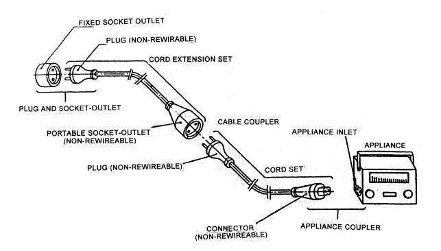
FIG. 59 PLUG SOCKET OUTLET AND ASSOCIATED ACCESSORIES
