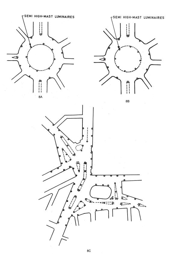
Fig. 8 Use of Semi-Mast or Conventional Lighting in Roundabouts (Three Alternatives)
