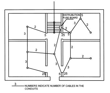
Fig. 52 Typical Arrangement of Concealed Conduits Feeding Lighting Points by Looping the Conduit into the Back of Outlet Boxes
