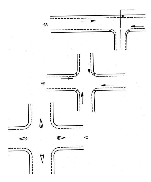
• = Locations of Columns Fig. 4 Simple Two Road Junctions (Three Alternatives)
