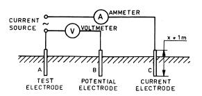
Fig. 5 Method of Measurement of Earth Electrode Resistance
