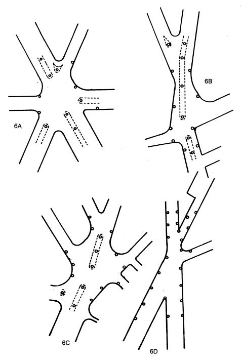
FIG. 6 MULTIPLE ROAD JUNCTIONS (FOUR ALTERNATIVES)
