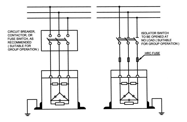
Fig. 2 Methods of Connecting Capacitors to Supply Line for Improvement of Power Factor
