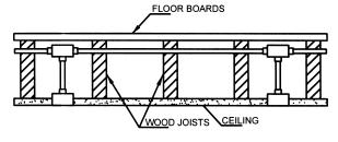
Fig. 51 Running Conduit in Wood Floors to Feed Lighting Points
