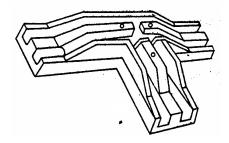
FIG. 23 T-JOINT OF CASING WITH BRIDGES
