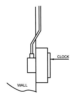
FIG. 50 SURFACE CONDUIT SYSTEM WHEN FITTING/ Accessory must be Flush on Wall or Ceiling
