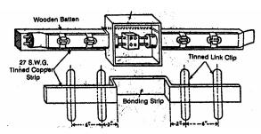
Fig. 29 Use of Bonding Metal Strip in a Wooden Joint-box
