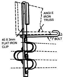
Fig. 43 Supporting Several Conduits from Angle Iron Truss
