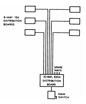
NOTE — It is recommended that distribution boards located remote from main switchgear be provided with local isolators.
