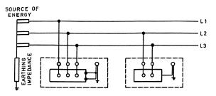
NOTE — All exposed conductive parts of an installation are connected to an earth electrode.
