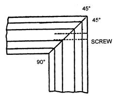
Fig. 17 Joint at a Corner
