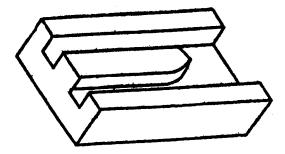
Fig. 25 Cutting Off a Portion of Casing in Order to Fit it with a Wall-tube  $% \mathcal{F}(\mathcal{F})$
