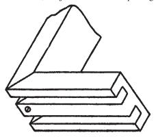
Fig. 20 Joint of Casing on the External Sides of Walls
