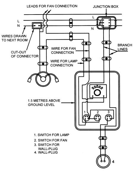
FIG. 12 AN EXAMPLE OF CLEAT WIRING SYSTEM
