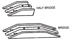
FIG. 22 HALF BRIDGE AND BRIDGE
