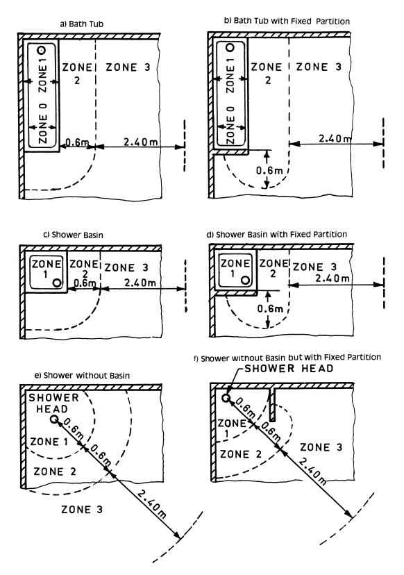
FIG. 2 ZONE DIMENSIONS (PLAN)
