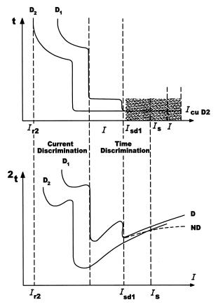
FIG. 21 DISCRIMINATION AT VARIOUS FAULT CURRENTS
