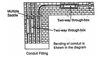
FIG. 33 BENDING OF CONDUIT
