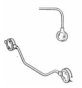
NOTE — Cable must not be drawn round more than two right angle bends or their equivalent. The four bends in the lower diagram are each  $45^{\circ}$  making a total of  $180^{\circ}$  in all.
