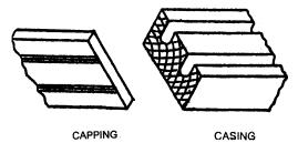
FIG.14 WOODEN CAPPING AND CASING
