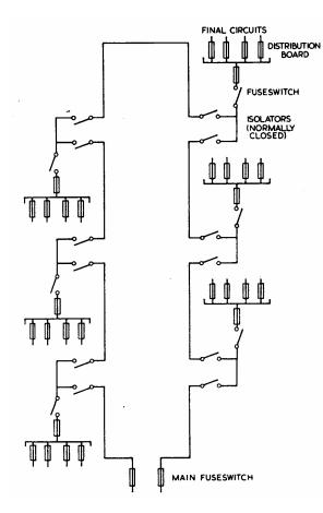
NOTE — The cables feeding the ring will share the load and may therefore be reduced accordingly. This arrangement enables the ring to be broken by one of the isolators in the event of a fault a one end of the ring, in which case the load must be reduced.
