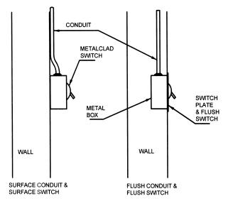
NOTE — At switch positions, conduit must terminate with metal box or other suitable enclosure.
