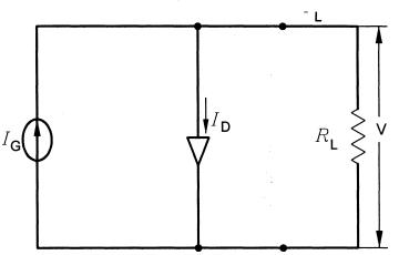
FIG. 4 CIRCUIT MODEL OF PV CELL
