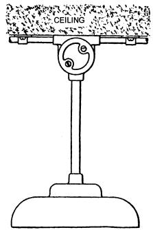
NOTE — The conduit is fixed to the ceiling with spacer bar saddles.
