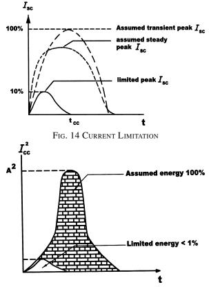
FIG. 15 THERMAL STRESS LIMITATION
