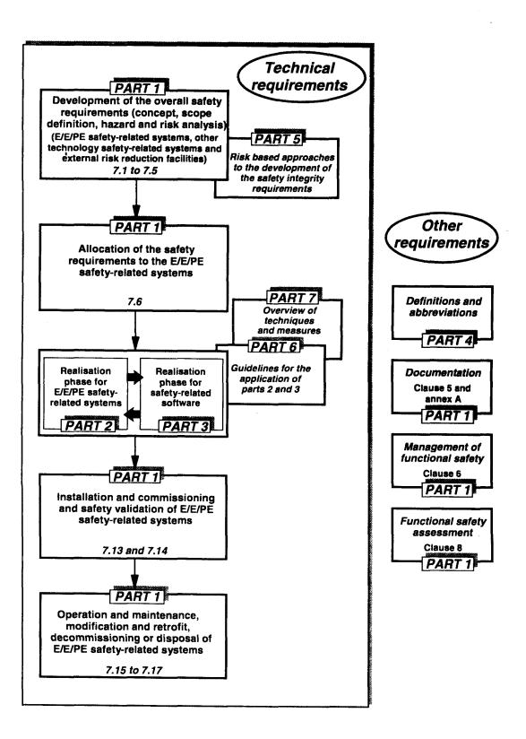
Figure 1 – Overall framework of IEC 61508
