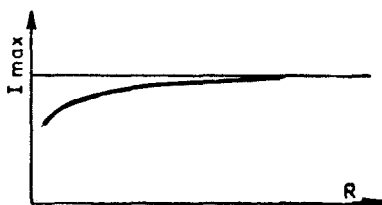
FIG. 3 APPARENT LUMINOUS INTENSITY CURVE DEPENDING ON MEASURING DISTANCE
