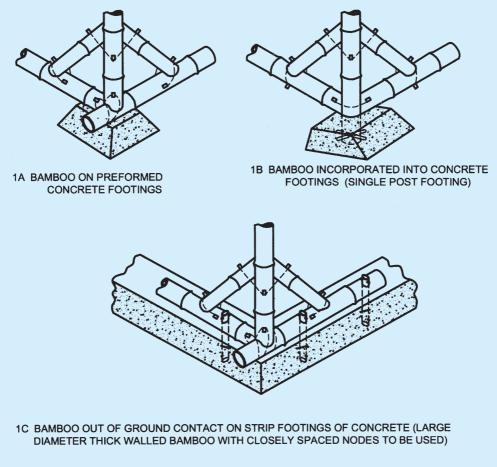
FIG. 1 BAMBOO FOUNDATIONS
