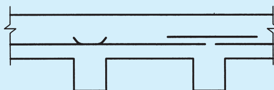
FIG. 3 ANCHORING OF TIES IN SLABS
