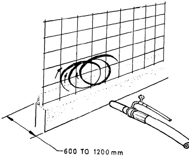
FIG. 1 CORRECT USE OF THE NOZZLE
