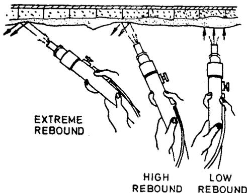
FIG. 5 EFFECT OF NOZZLE ANGLE ON REBOUND
