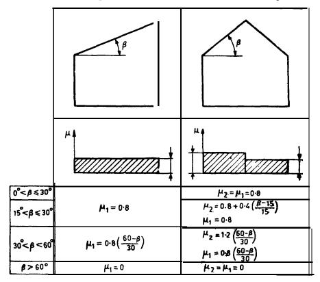
4.2.2 Simple or Multiple Pitched Roofs Two-Span or Multispan (Negative Roof Slope) Roofs
