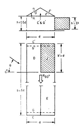
Roof slope  $\alpha = 30^{\circ}$ Effects of trains or stored materials:  $\theta = 0^{\circ} - 45^{\circ}$ , or  $135^{\circ} - 180^{\circ}$ , D, D', E, E' full length  $\theta = 90^{\circ}$ , D, D', E, E' part length b', thereafter  $C_{\mathbf{p}} = 0$
