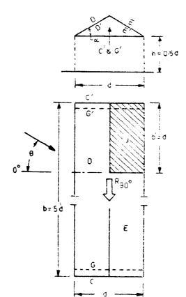
Roof slope  $\alpha = 30^{\circ}$   $\theta = 0^{\circ} - 45^{\circ}$ , D, D', E, E' full length  $\theta = 90^{\circ}$ , D, D', E, E' part length b', thereafter  $C_p = 0$
