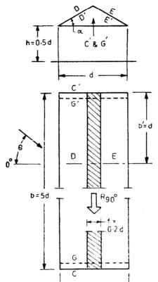
Roof slope  $\alpha = 10^{\circ}$   $\theta = 0^{\circ} - 45^{\circ}$ , D, D', E, E' full length  $\theta = 90^{\circ}$ , D, D', E, E' part length b', thereafter  $C_{\mathbf{p}} = 0$
