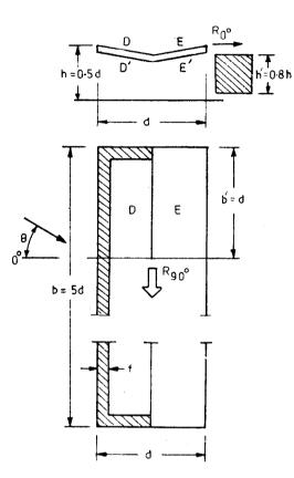
Roof slope  $\alpha = 10^{\circ}$ Effects of trains or stored materials:  $\theta = 0^{\circ} - 45^{\circ}$ , or  $135^{\circ} - 180^{\circ}$ , D, D', E, E' full length  $\theta = 90^{\circ}$ , D, D', E, E', part length b' thereafter  $C_{\rm P} = 0$
