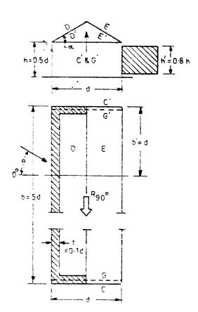
Roof slope  $\alpha=10^{\circ}$ Effects of trains or stored materials:  $\theta=0^{\circ}-45^{\circ}$ , or  $135^{\circ}-180^{\circ}$ , D,D',E,E' full length  $\theta=90^{\circ}$ , D,D',E,E' part length b', thereafter  $C_{\rm D}=0$
