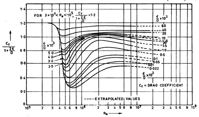
Fig. 5 Variation of  $\frac{C_{\rm f}}{1+\frac{2\epsilon}{D}}$  with  $R_{\rm e}$  (>3×10<sup>4</sup>) for Circular Sections
