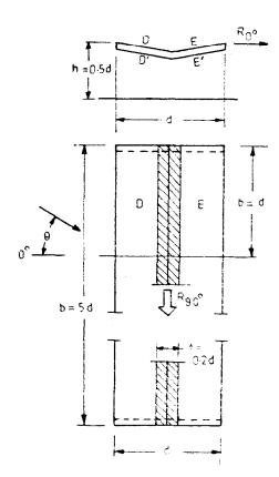
Roof slope  $\alpha = 10^{\circ}$   $\theta = 0^{\circ} - 45^{\circ}$ , D. D', E, E' fullingth  $\theta = 90^{\circ}$ , D. D', E, E' part length b', thereafter  $C_p = 0$
