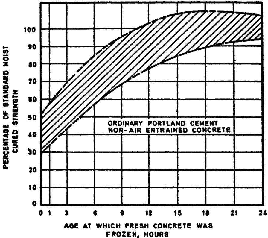
FIG. 3 EFFECT OF EARLY FREEZING OF CONCRETE
