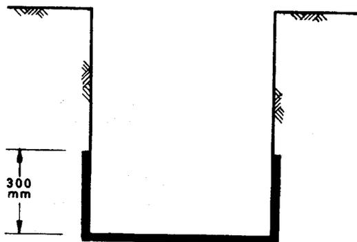
FIG. 1 TREATMENT OF TRENCH BOTTOM AND SIDES
