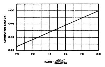
FIG 1 CORRECTION FACTOR FOR HEIGHT/DIAMETER MATIO OF A CORR.
