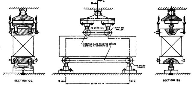
FIG. 3 ARRANGEMENT FOR LOADING OF FLEXURE TEST SPECIMEN
