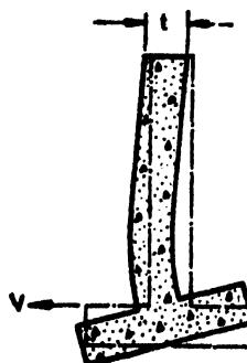
FIG. 7 WALL WITH SHEAR APPLIED AT BASE
