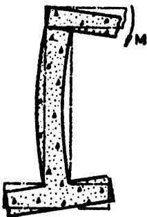
**FIG. 8 WALL WITH MOMENT APPLIED AT TOP**
