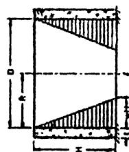
$T = \text{Coefficient} \times \omega H R \text{ kg/m}$
