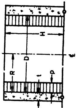
$t = \text{Coefficient} \times \rho R \text{ kg/m}$
