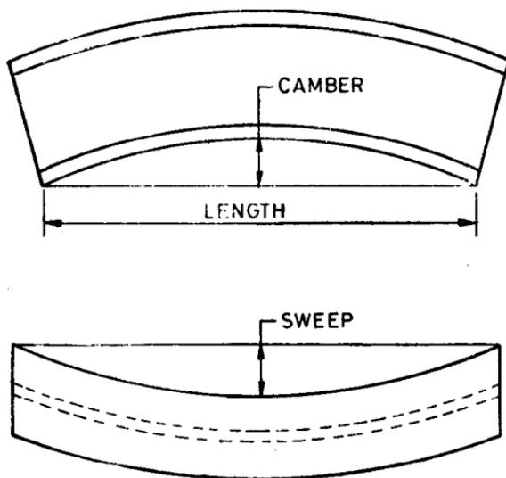
FIG. 3 MEASUREMENT OF CAMBER AND SWEEP
