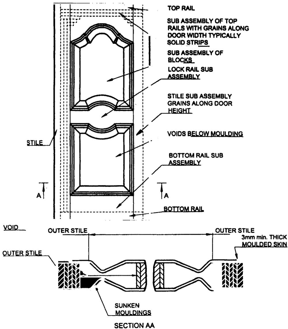
FIG. 2 TYPICAL MOULDED RAISED HDF PANEL DOOR
