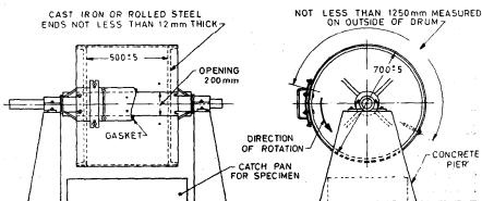
Note - Shaft bearing shall be mounted on concrete piers or other rigid supports.
