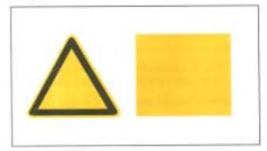
FIG. 12 LAYOUT FOR A COMBINATION SIGN WITH THE SUPPLEMENTARY SIGN TO THE RIGHT OF THE SAFETY SIGN.
