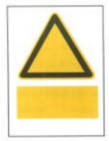
FIG. 11 LAYOUT FOR A COMBINATION SIGN WITH THE SUPPLEMENTARY SIGN BELOW THE SAFETY SIGN
