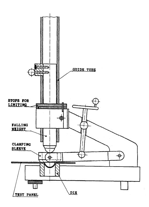
Fig. 2 Side-View of Falling-Weight Apparatus
