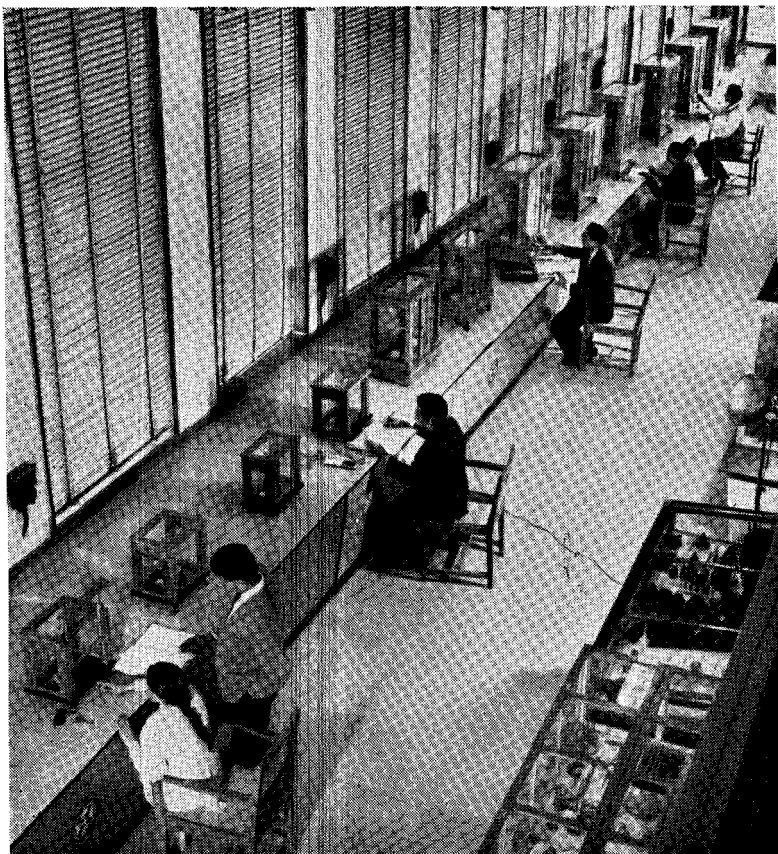
Testing at NPL, New Delhi, of secondary standard balances for use by weights and measures enforcement departments
