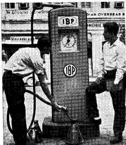
A dispensing pump with a moving dial indicator which required only re-calibration and no additional gear mechanism to register in litres
