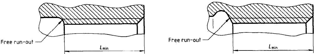
Figure 4 — Internal threads with free run-out
