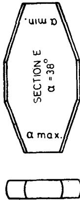
FIG. 4 LIMIT GAUGE FOR GROOVE ANGLE
