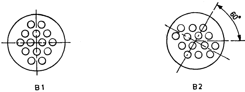
FIG. 9 FLOW CONDITIONER TO DAMP OUT HIGH LEVEL PERTURBATION
