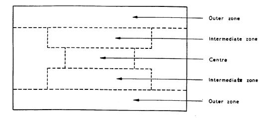
Figure B.1 — Diagram showing cutting for moisture determination
